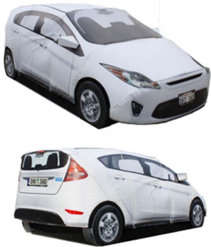
Figure 4. Global Vehicle Target (GVT) according to ISO 19602 Part 1
