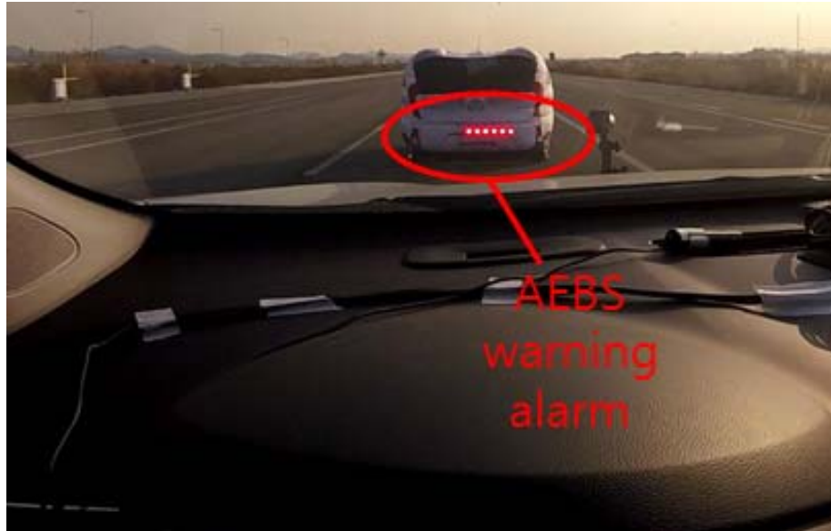
Figure 5. AEBS warning test of 3D balloon dummy car
