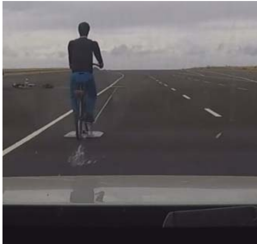
Figure 12. Example of ACC longitudinal VRU test scenario
