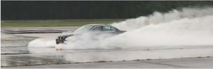
Figure 13. Hydroplaning assistance vehicle test at the “Contidrom” proving ground with front wheels floating. The vehicle is controllable by rear wheel brake torque vectoring
