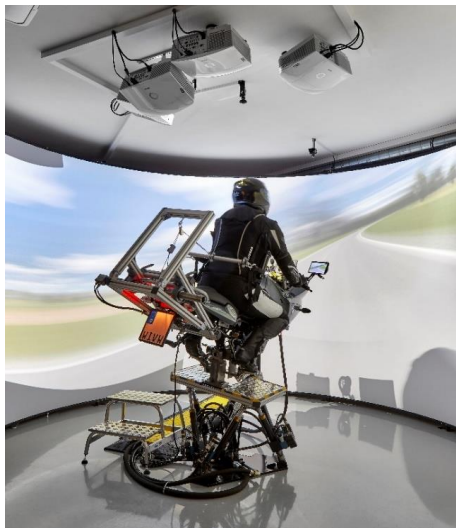
Figure 4. DESMORI Dynamic Motorcycle Riding Simulator at WIVW
