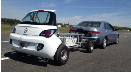
Figure 3. Dummy target EVITA
