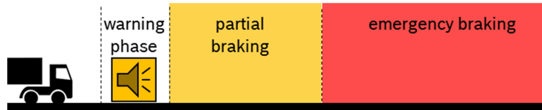
Figure 4: Schematic view of AEBS phases
