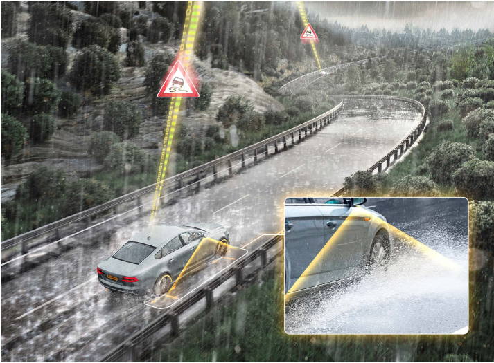
Figure 7. Water spray detected by surround view cameras for vehicle near field sensing
